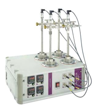
The "ROFOX four" from the ROFOX series is a compact and automatic Oxidation Stability Tester with 4 independent test positions.
