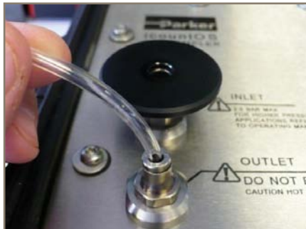
Attach OUTLET (Ø 4mm) hose
